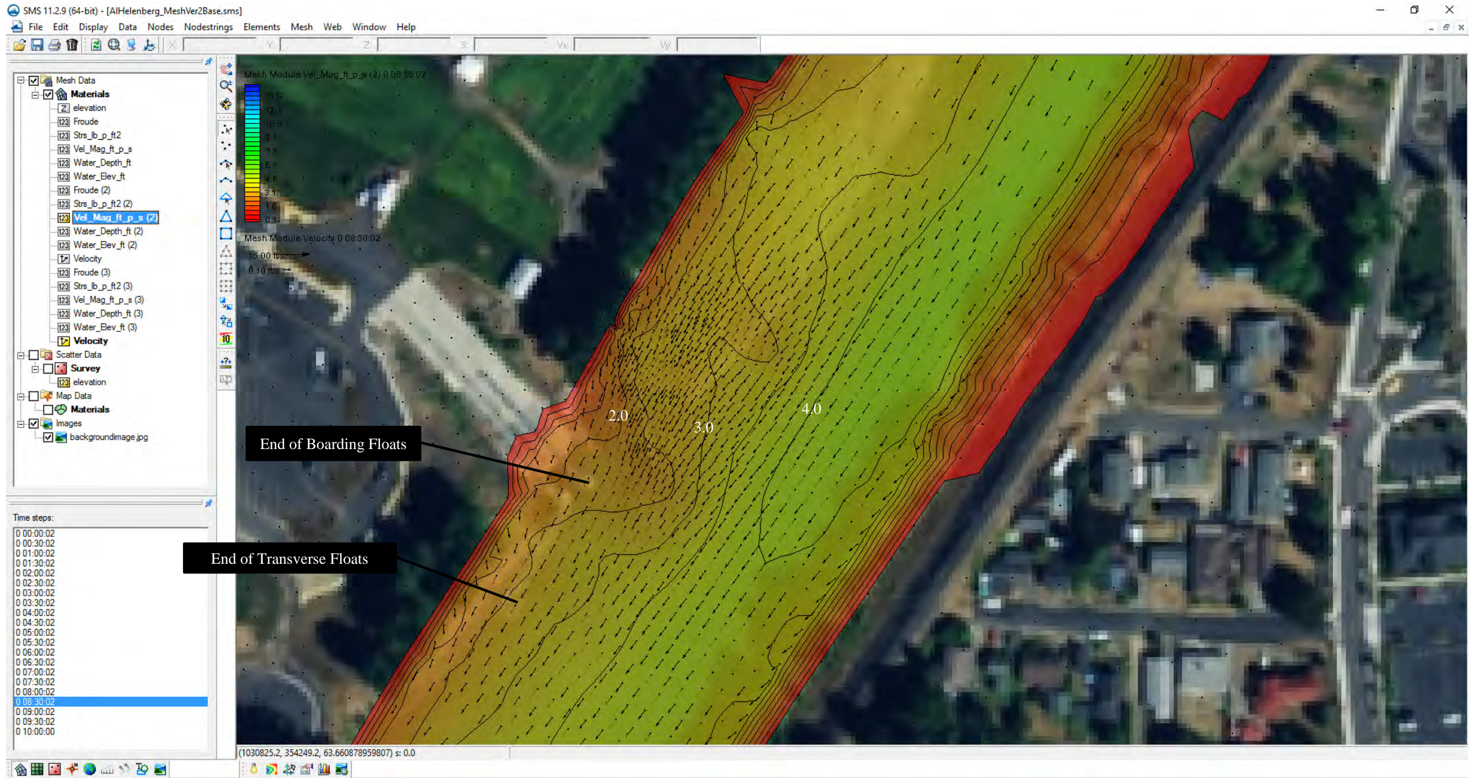
Figure 5. Existing conditions velocities (9,000 cfs)
